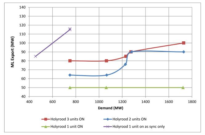
Figure 5-7. ML export limits, 2 SOP synchronous condensers in-service
