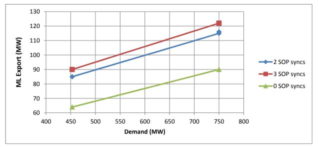
Figure 1-2. Island demand < 750 MW. Maximum ML export levels - 2 (blue), 3 (red) and 0 (green) SOP synchronous
