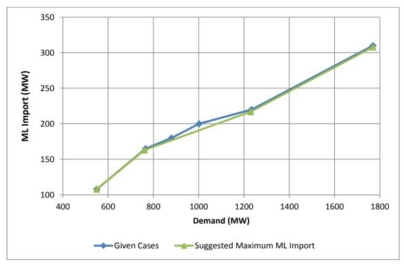
Figure 5-5. ML import limits, no synchronous condensers in-service
