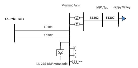
Figure 3-2. Labrador system near Muskrat Falls
