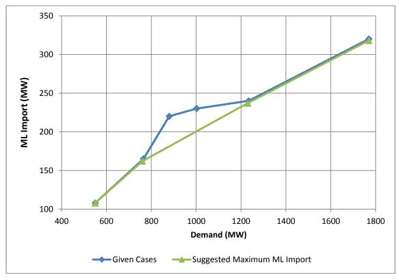
Figure 5-3. ML import limits, 2 SOP synchronous condensers in-service
