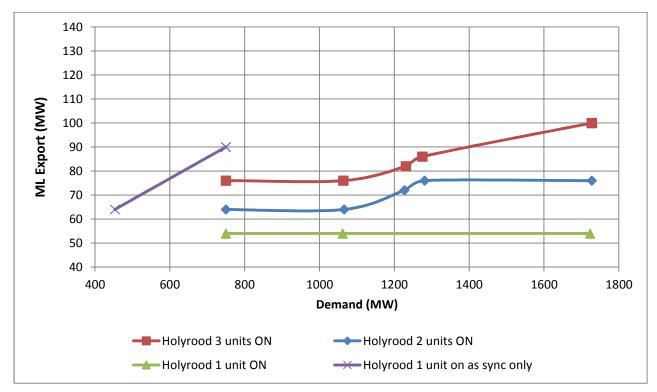
Figure 5-9. ML export limits, 0 SOP synchronous condensers in-service
